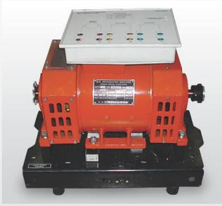
**Voltage:**  $V_{arm} = 180V$   $V_{field} = 180V$
