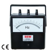
The Hz meters use a frequency-to-DC current transducer which drives a high sensitivity moving coil type indicator. It features accurate frequency measurements without noticeable influence of line voltage fluctuation (50 to 300V) or waveform distortion.
