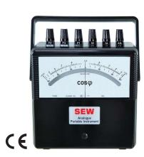
The PF meter is used for measurement in single-phase and balanced three-phase circuits. From a phase discriminating circuits, the output of the built-in transducer produces a DC proportional to the phase between voltage and current to operate the DC indicator.
